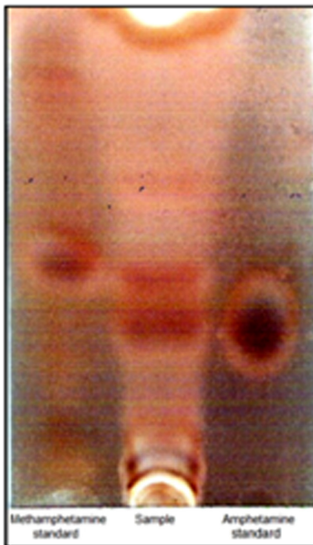
Figure 3. Chromatogram shows the spot(s) of the amphetamine and methamphetamine standard and a urine sample containing both of them.
